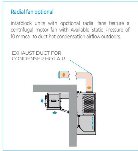
230V/400V 50Hz | Positive temperature | Hermetic compressor | R-290
